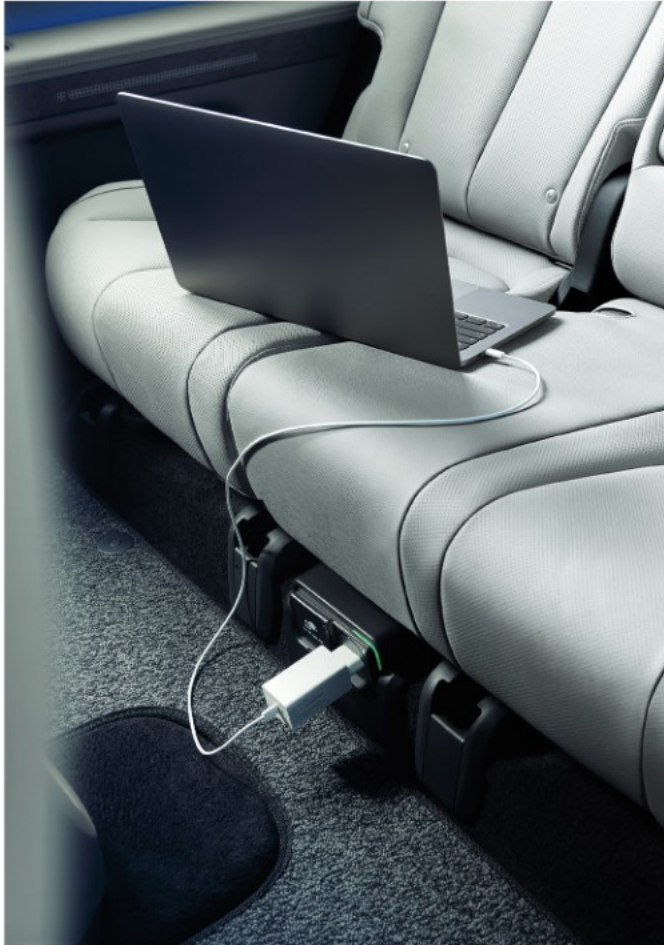
Vehicle-to-Load (Inside V2L)
